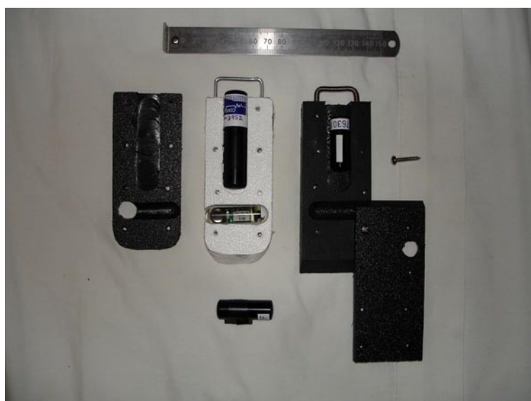
Photo: Close up of the sonic locator and depth recording unit.
